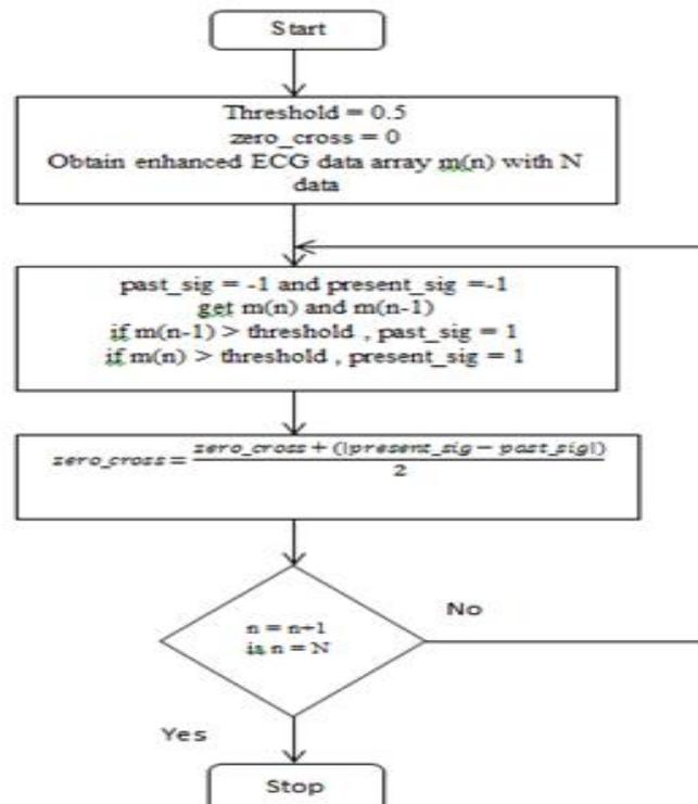
Fig. 5: Zero cross algorithm
