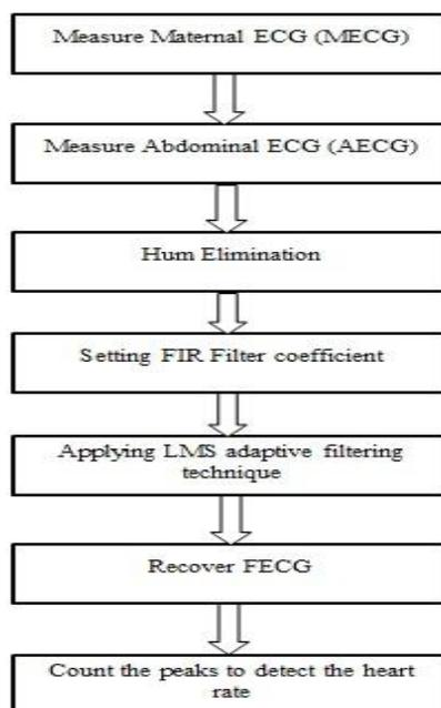
**Fig. 2:** Flow diagram representation
